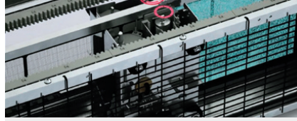
Cleaning unit moves across the filter removing dust which is collected in the dust box
